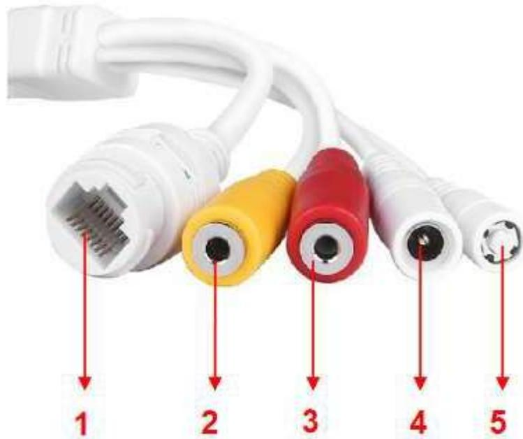
1. LAN 10/100M adaptive Ethernet interface. Through this interface, IP camera can relate to various network devices, such as hub, router, etc.
