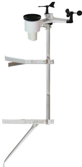
The EZ-30-12 mounting pole kit provides a stable weather station mounting solution, ideal for mounting to a vertical wall, chimney, eave, or fence post.
